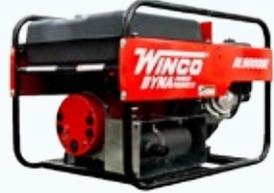
Generators can be either temporary or permanently installed. A permanent generator is wired into a house by a qualified electrician, using a transfer switch that prevents a generator from feeding electricity back into overhead lines, which can be deadly for linemen. A temporary generator should not be attached to a circuit breaker, fuse or outlet.
